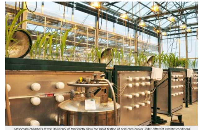
Mesocosm chambers at the University of Minnesota allow the rapid testing of how corn grows under different climatic conditions
